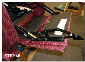
STEP 6 – Remove (2) 1 1/2" bolts, small spacers, and lock nuts from the kit. Insert each bolt through the scissor mechanism. Place a spacer on each bolt, align the holes in the bracket and insert the bolts. Place a lock nut on each bolt and tighten to secure. See figure 6B for completed assembly. Repeat for opposite side.
